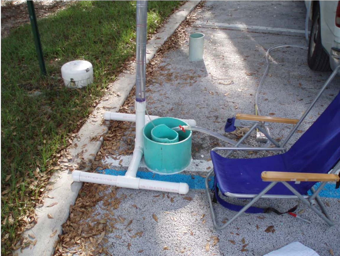
Figure 5.2 - Embedded Ring Infiltrometer Kit (ERIK) Showing On-Site Measurement
